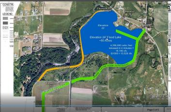
Also showed essential elements of Phase 2 (left aerial), and what could occur if both levees (Corps dike and Phase 1 levee) remain in place during flood season (right aerial). Water that gets between the levees would pond up and create a lake, and potential catastrophic flooding. Removing the Corps dike would prevent that. Randy estimated that removing the Corps dike could take two to four weeks.
